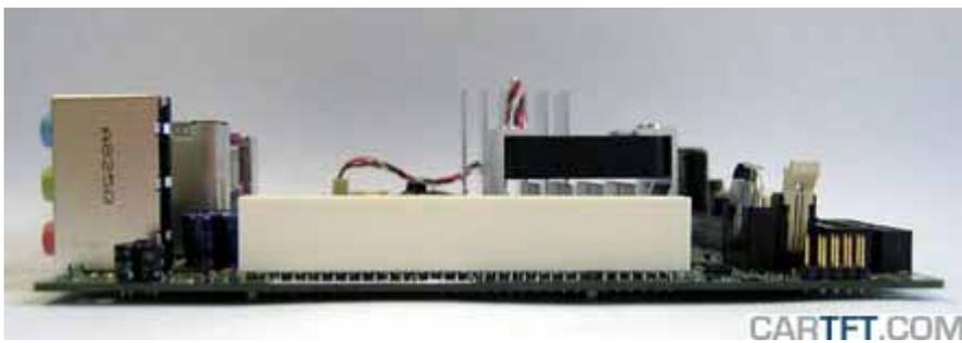
CarTFT.com offers an replacement heatsink for the D945GCLF, which fits onto the D945GLCF2 so the board fits into the most usual mini ITX enclosures, too.
